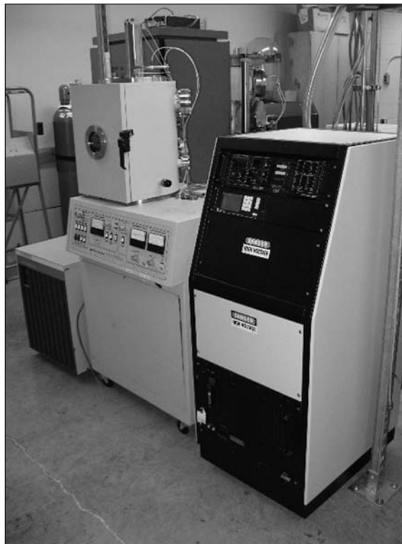
A Denton electron beam evaporator system replaces an aging Veeco thermal evaporator with improved process control.
