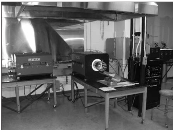
An additional Mellen 3-zone benchtop furnace was installed and characterized for dopant diffusion during 2009.
